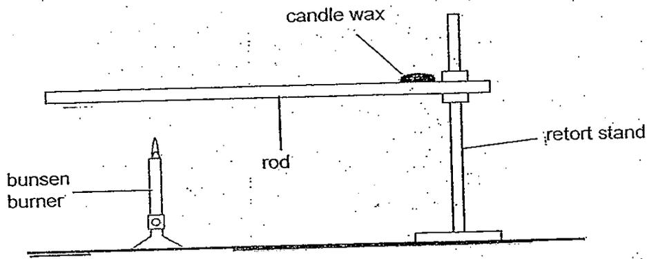
The time taken for the candle wax on each rod to melt completely is recorded as shown in the table below.
